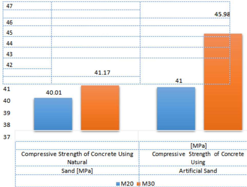
Figure 2 Compressive strength of concrete
