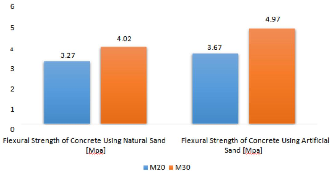
Figure 3 Flexural strength of concrete
